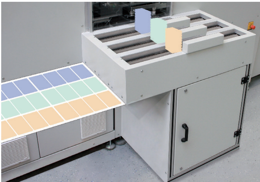
Sorting option S3L: Sorting by "columns"; all cards punched by one punching tool/die are stacked into individual magazines.
