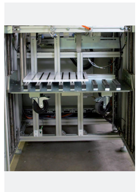
Trolleys for stacking the sheets outside of the machine allowing fast reloading.
